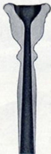
6042 Del Staigers' Model, for trumpet. Spectral design. Medium cup, medium bore, soft cushion rim.
